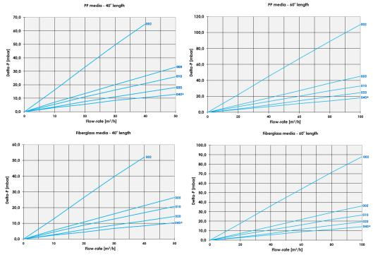
Flow-rate valid for clean water, reduce the flow-rate according to the application. Delta-P valid for 1 cP viscosity liquids; for different viscosity, multiply the indicated Delta-P by the fluid viscosity in cP. For total assembly filter Delta-P, the filter housing Delta-P must be always added.
